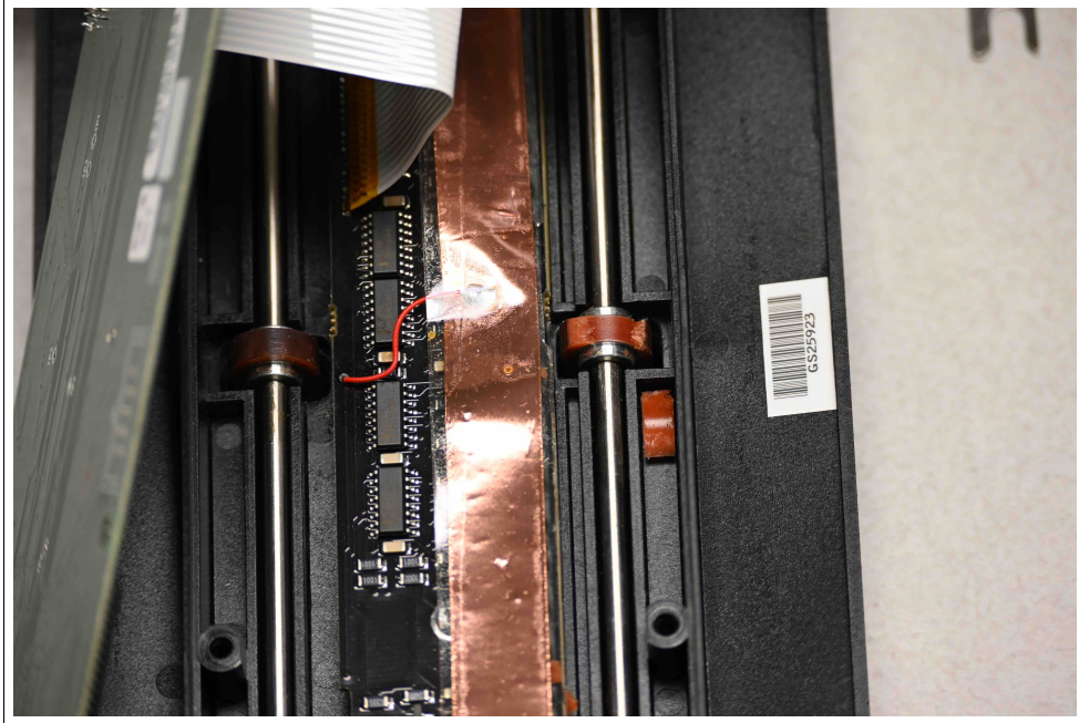
Figure 6. Damaged roller missing a large fragment.
